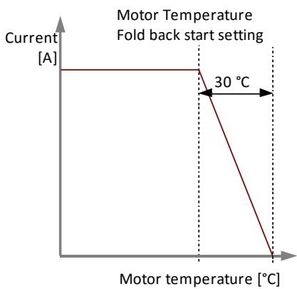
The maximum current value is rolled back as soon as the motor temperature is above its starting point adjustment (parameter 2 in the limits setup menu). It is cut back proportionally between the starting point and 30 °C above the starting point as shown in the graph below.
